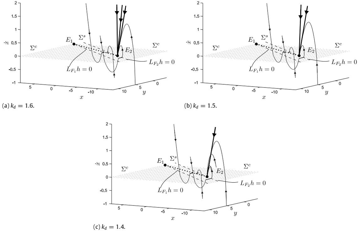
**Fig. 7.** System (19) with  $c = 0.5$ ,  $k_p = 1$  and  $F_s = 2$ , showing a bifurcation near the endpoints at  $k_d = 1.5$ . The equilibrium set  $\mathcal{E}$  is given by a dotted line, and the real eigenvectors of  $A_2$  are represented with thick lines.
