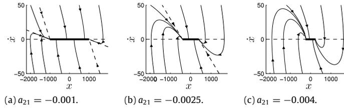
**Fig. 3.** System (14) with  $F_s = 1$  and  $a_{22} = -0.1$  showing a focus-node bifurcation. The equilibrium set  $\mathcal{E}$  is given by a bold line, the real eigenvectors of the stable eigenvalues of  $A$  are represented with dashed lines. The real eigenvectors are distinct for  $a_{21} > -0.0025$ , collide at  $a_{21}$  and subsequently become imaginary.
