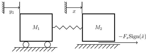
Fig. 1. Mechanical system subject to dry friction.
