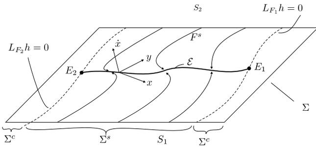
Fig. 2. Sketch of discontinuity surface  $\Sigma$  of (2)–(6) with  $n = 3$  and  $F_s > 0$ , containing an equilibrium set  $\mathcal{E}$ .
