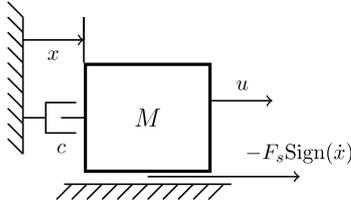
Fig. 6. Example of mechanical system subject to dry friction.
