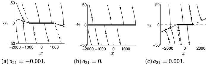
**Fig. 5.** System (14) with  $F_s = 1$ ,  $a_{22} = -0.1$  and varying  $a_{21}$ , showing a bifurcation when an eigenvalue becomes zero and the system is linear. The equilibrium set  $\mathcal{E}$  is given by a bold line, the stable or unstable manifolds are represented with dashed lines. At  $a_{21} = 0$ , the equilibrium set coincides with the line  $x \in \mathbb{R}, \dot{x} = 0$ .
